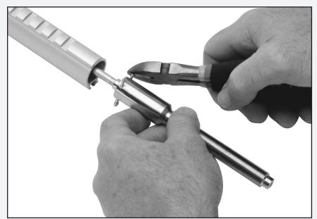
Assemble turnbuckle and attach Harken toggle.
