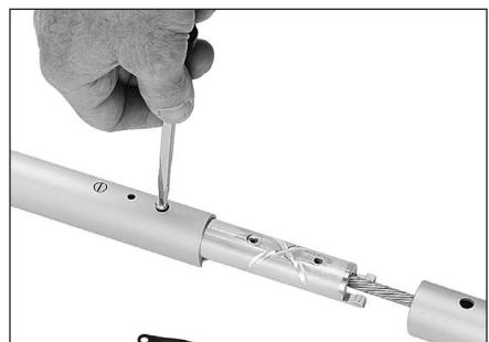
Use bushings, connector, wedge and adhesive in other screw hole and insert into other foil. Use 3/4 - 1ml of adhesive.
