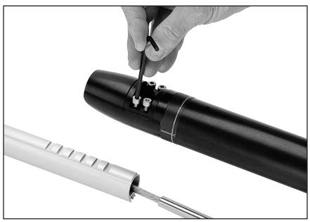
Slide drum assembly onto foils.
