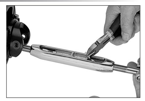
Slide lower drum assembly over turnbuckle and attach using long crosspin.
