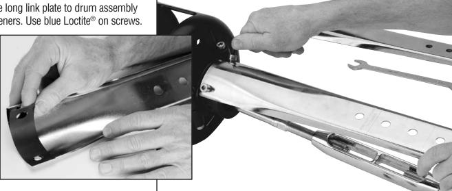
Fasten second long link plate to drum assembly and secure to clevis pin using locknuts.
