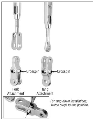
Most boats have a chainplate with a single tang. If boat has two plates forming a jaw, reverse eye/ jaw toggle so eye is down.
