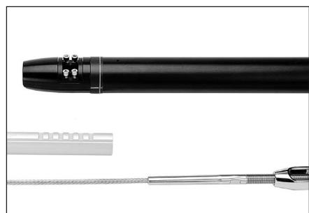
**Note:** Position top foil so that with top cap the foil will ride 5/8" (16mm) below terminal. If wire fitting at top of stay is swage, foil must ride just below shoulder of swage. Mark cut line on foil. Wrap tape around foil as a guide so cut is straight.
